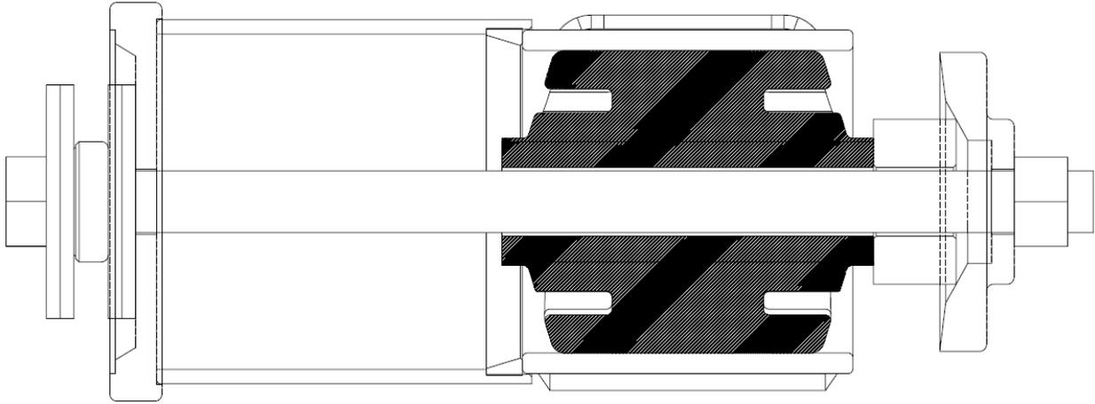
Figure 3 (Bushing in Arm sleeve before removal)
