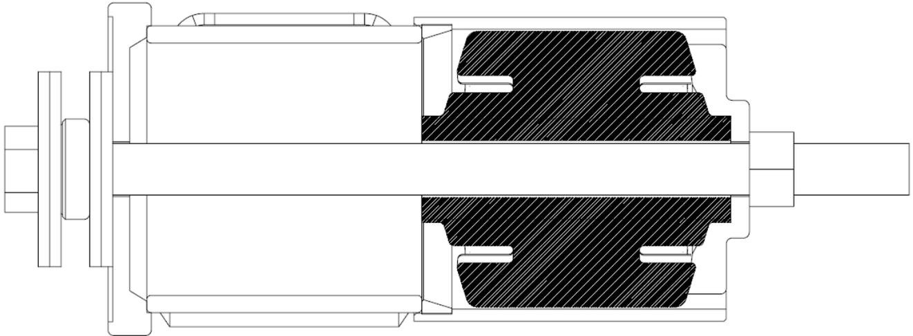
Figure 5 Bushing in Transition Tube before installation
